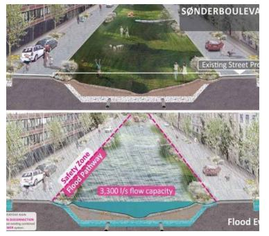
Green infrastructure can be created in multi-functional spaces that can be used for recreation in dry weather, but provide flood storage in extreme weather. Source: Ramboll
